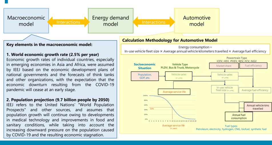
Figures for future fuel consumption (CO<sub>2</sub> emissions) were calculated using IEEJ's macroeconomic model and energy demand model reflecting JAMA's powertrain mix estimates.
