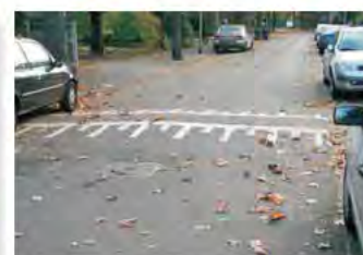
Speed inhibitors (speed bumps) form a small change in vertical alignment while maintaining surface grip, so can be safe for the PTW rider (source: DTV Consultants, the NL).
